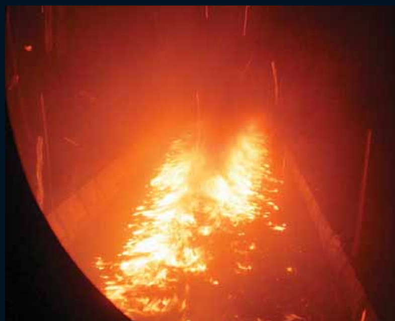
Fig. 2 Post-combustion of RDF residue on the MAP® -Belt
