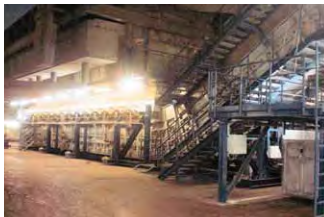
Fig. 3 MAP® - Post-combustor on rails
