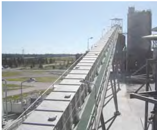
150m long Magaldi Ecobelt® conveyor in Millmerran Power Station for ash transportation.
