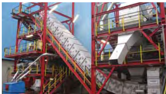
A 45° inclined Magaldi Ecobelt® conveyor in Venice Fusina Power Station.
