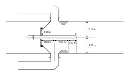
The height of the dam ring is to be considered at a later time, but normally app. 0.35 to 0.45 m over the kiln lining as the original refractory drawing shows.
